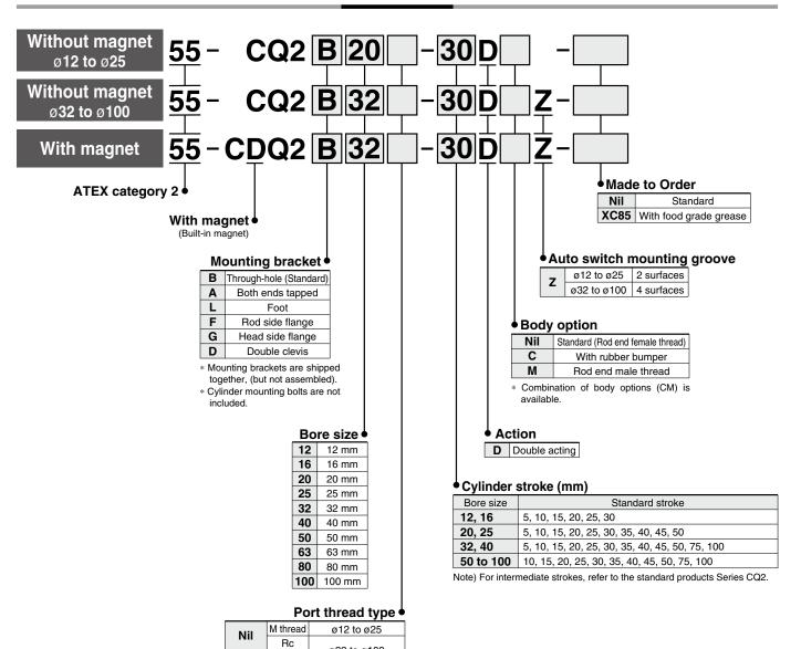
\* For cylinders without magnet, M threads are compatible only with ø32-5 mm stroke.
