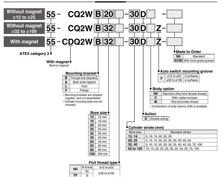
\* For cylinders without magnet, M threads are compatible only with ø32-5 mm stroke.
